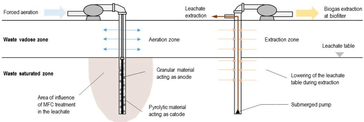
Figure 2. Representation of the scheme of application of the two technologies (microbial fuel cells and in-situ aeration) to landfill.
