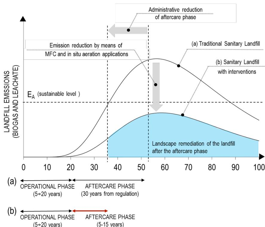
Figure 1. Long-term emissions for a traditional sanitary landfill (a) and for a sanitary landfill where new technologies for the achievement of sustainability ( $E_A$ ) within the aftercare phase are
